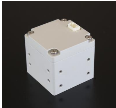
ASPINA "Ultra-compact reaction wheel for CubeSat"
